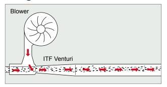
With this system the Venturi is installed nearby the pick-up location where the material originates.
